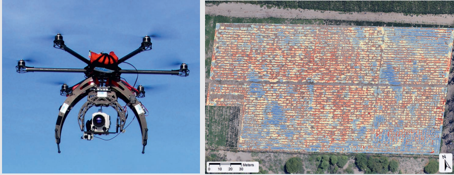
Figure 33.1. A. A hexacopter equipped with a camera and a thermal camera. B. A hyper-resolution mapping of the surface temperature of the canopy, only of sweet potatoes.
